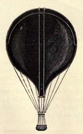
VALVES are fitted at the neck and at the top of a balloon.
